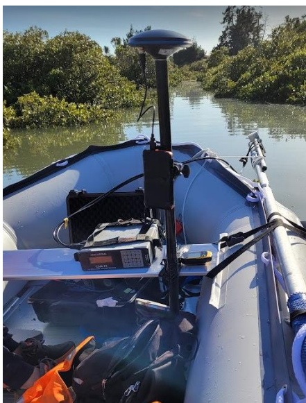
(Above) Magnetometer and SBP surveys in progress, Pakuranga Creek.
