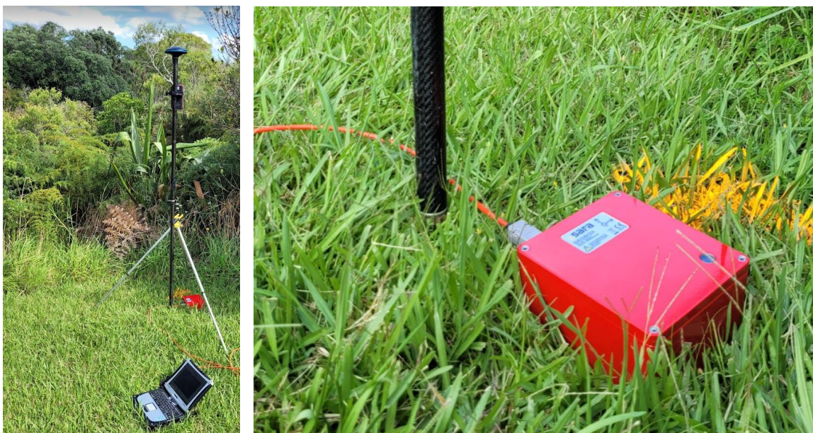
(Above) HVSR equipment in use. Seismograph has 3 long stainless steel spikes which are pushed into ground to couple with soil.
